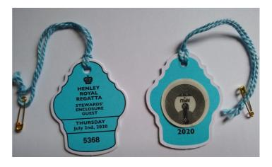
The UHF Tags that the antenna were reading comprised of a cardboard lapel badge with a UHF Label with an adhesive backing attached to the reverse side. The scanning antenna were calibrated to read the Tags from a couple of metres. This ensured accurate scanning of those arriving and departing but not scanning a Tag several metres away, unrelated to the access points.
